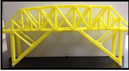
You will work with a group of up to three people to construct a bridge that will span a 35.0 cm gap. The bridge needs to be no longer than 45.0 cm but it must be longer than 35.0 cm or it will fall into the crevasse. The roadway must be at least 5 cm wide for traffic to cross. To the right, you see one that held 5200 g or about 11.4 lbs and had a finished mass of only 32 g (just over an ounce!)
